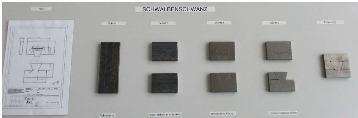
Picture 1.: Visualisation of a typical workpiece (dovetail joint) in the first year of AVL technical apprentices.
